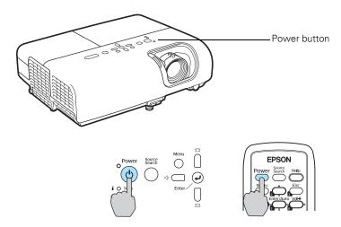
The projector beeps and the power light flashes green as the projector warms up. The projector lamp comes on in about 4 seconds and the power light stays green.
