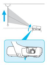
Once the image is positioned where you want, release the lever to lock the foot in position.
