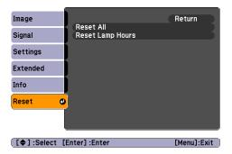
To reset most projector menu settings, select Reset AII and press the Enter button to display the confirmation screen. Select Yes to reset all the default settings or No to cancel.
