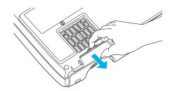
4. Align the new filter carefully as you slide it into place. It should click into place.
