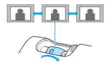
Press the Wide button on the projector to enlarge the image, or the Tele button to reduce it.
