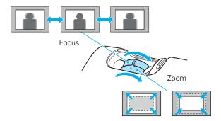
You can also change the image size by moving the projector closer to or farther away from the screen. You can use the E-Zoom buttons on the remote control to zoom in on a portion of the image. See page 47 for instructions.
