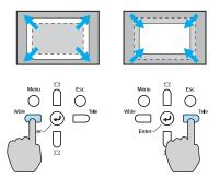
You can also change the image size by moving the projector closer to or farther away from the screen. You can use the E-Zoom buttons on the remote control to zoom in on a portion of the image. See page 47 for instructions.
