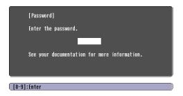
Use the numeric buttons on the remote control to enter the password. Once you have entered the password correctly, the password screen closes, and projection begins.
