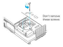
6. Hold the lamp as shown and pull it straight out.
