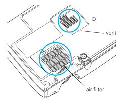
If the dirt is difficult to remove or if the filter is torn, replace it. Contact your dealer or call Epson at (800) 463-7766 to obtain a new one (part number V13H134A13).
