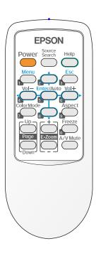
The remote control lets you access your projector's features from anywhere in the room—up to 20 feet away. For example, you can turn the projector on and off, freeze the presentation, zoom in on a portion of your image, and access the menu system. (The projector menus let you adjust many projector settings; see Chapter 4.)
